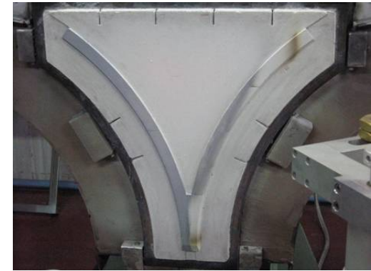
Side dams for twin roll strip caster
