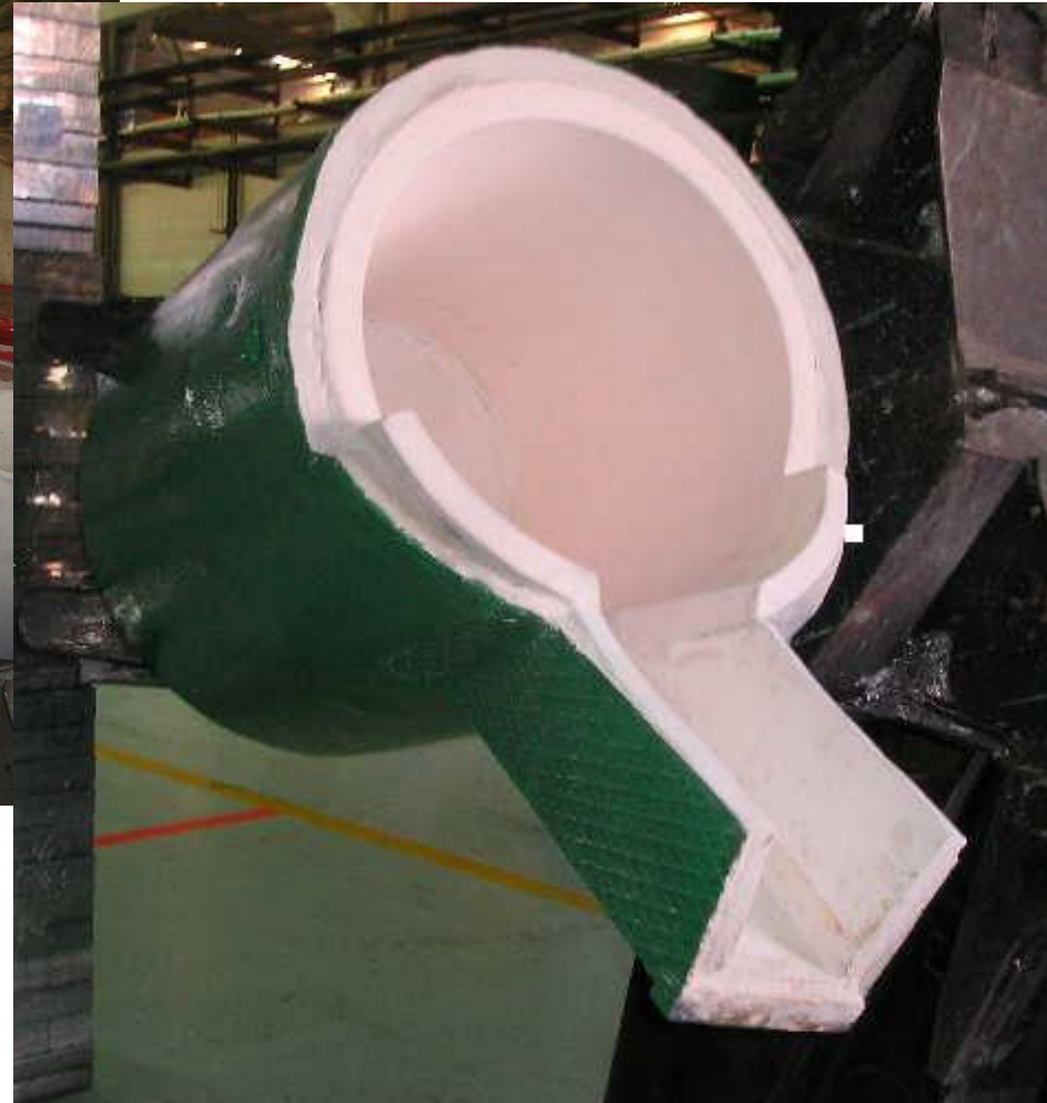
Refractory ladle: After Insural ATL 600
