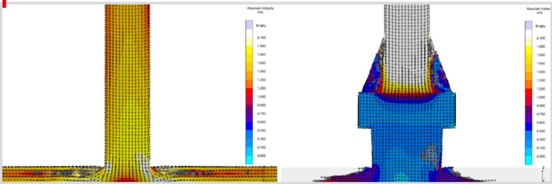
Fig. 4. Runner Bar Side Centerline Flow Comparison for No Filter and Standard Filter Print Gating at 0.9 Seconds
