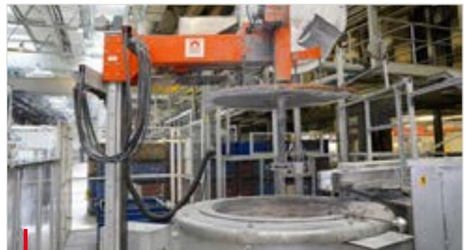
SMARTT process control for rotor degassing of molten aluminium
