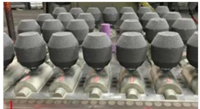
Pattern plate with FEEDEX HD1 VAK 159/61M sleeves
