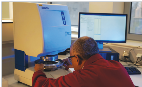
Powder Flow Tester for the determination of the sand flowability
