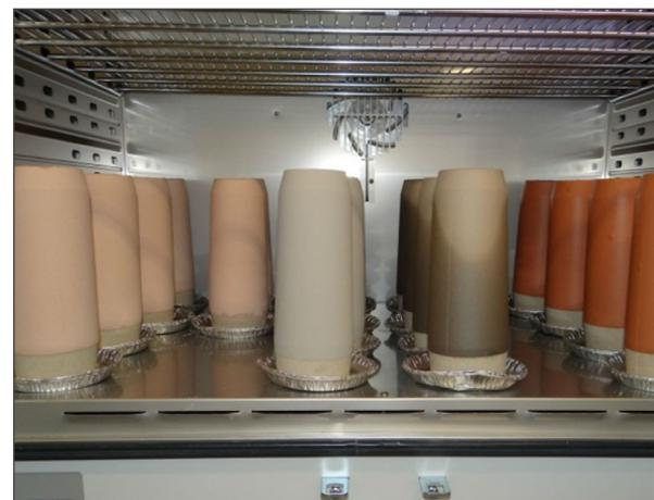
(a) Drying coated cores in an oven
