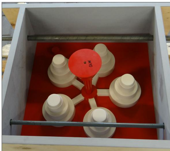
Figure 7. Casting layout and the tooling used to produce the castings
