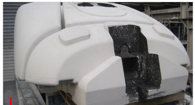
Finished core – 50% faster supplied to moulding line
