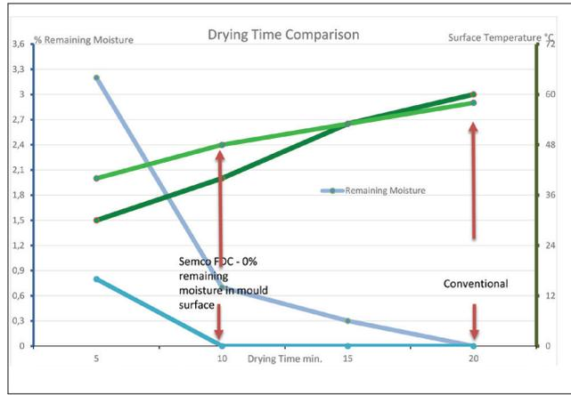
Figure 3. Remaining moisture and surface temperature versus drying time of two different coatings
