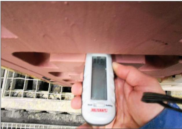
Figure 2. Checking surface temperature of the coated mould
