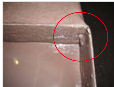
Figure 2. Coating remains unmixed in dead areas in dip tank
