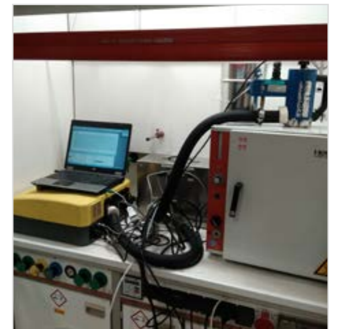
Figure 5. FTIR test set up
