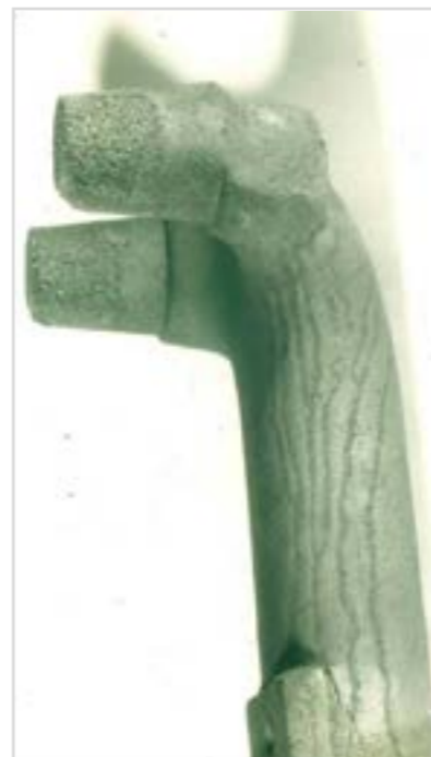
Figure 3. Syneresis when applying bacteria affected coating
