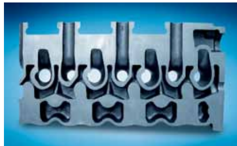
Figure 1 Complex internal passages of a cylinder head
