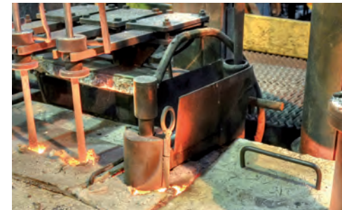
For most ferrous foundry installations, simple mounting brackets keep the system in position. The probe and protector tube can be changed easily
