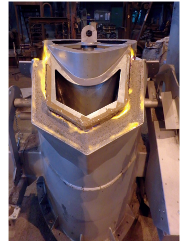
INITEK ISO granular refractory lining installation and exothermic set
