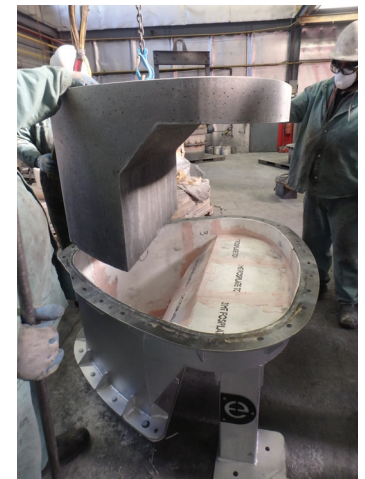
INITEK ISO granular refractory lining installation and exothermic set
