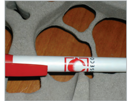
Completely compacted core bridges of a water jacket core produced with SOLOSIL TX for an aluminium cylinder head for a passenger car
