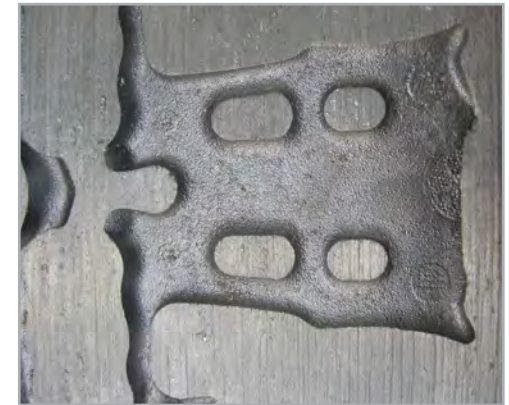
By successful development of the SOLOSIL TX additive it was possible to eliminate the metal-sand reaction completely
