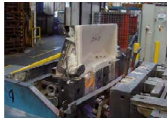
Pouring basin to fill the mould
