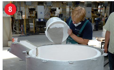
The gap is filled with the rest of the backing material up to the top, it is compacted and sealed with a layer of INSURAL 800 mastic of approx. 15 mm
