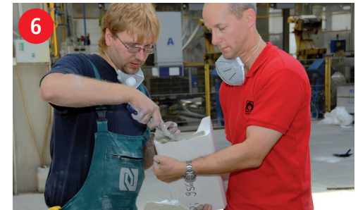
INSURAL 800 mastic is applied to the spout
