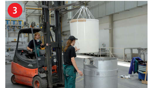
Inserting ATL lining in the steel shell
