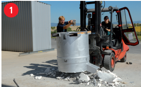
Easy removal of old lining
