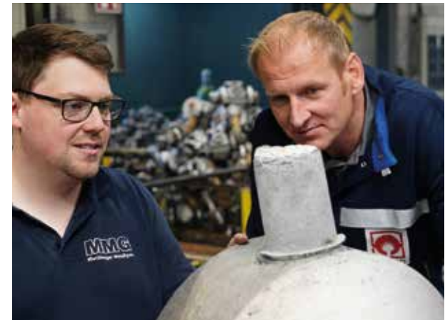
Riser ready to be knocked off after casting
