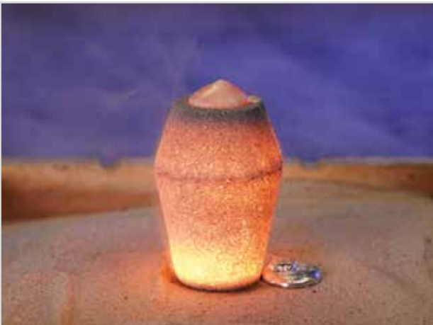
Figure 4. Constant burn-off of the FEEDEX NF1 feeder
