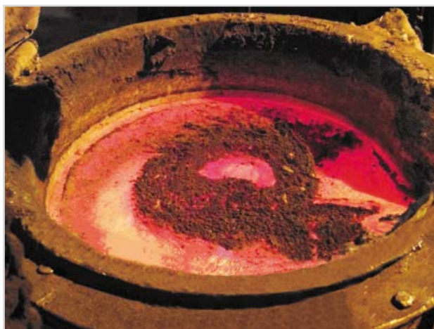
Figure 11: Photograph of extremely dry dross in transfer ladle after treatment with COVERAL MTS 1582.
