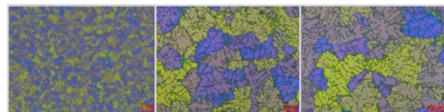
Figure 9b: After treatment. Grain size d_m [ \mu\text{m} ] = 206
