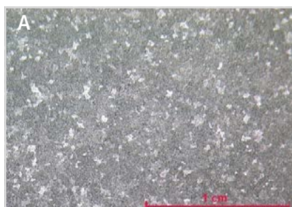
Figure 10: Comparison of TiB rods with Coveral MTS 1582: grain size
