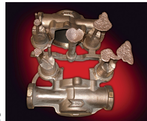
Casting made with Foseco sleeves
