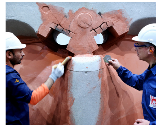
Brush coating designed to improve surface finish
