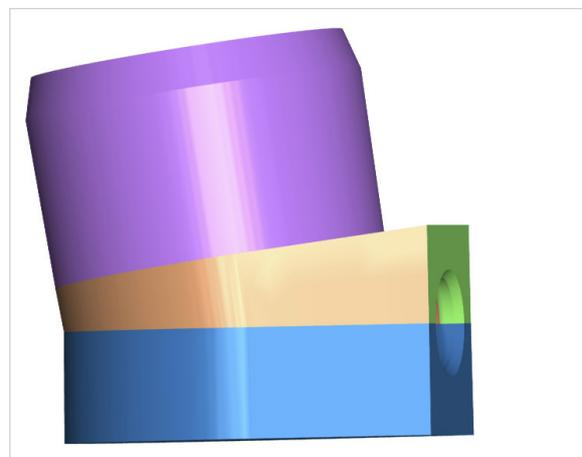
Figure 7. Feeder base with top part – 6.5 cm modulus
