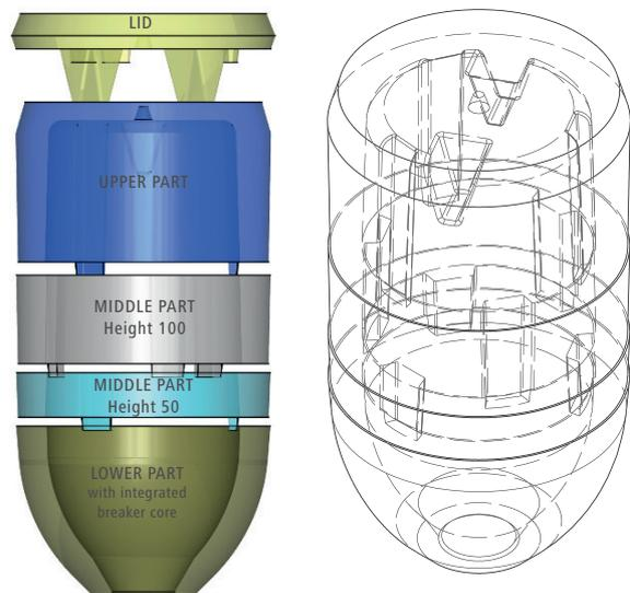
Figure 4. Modular construction – system diagram (left), wire model (right)
