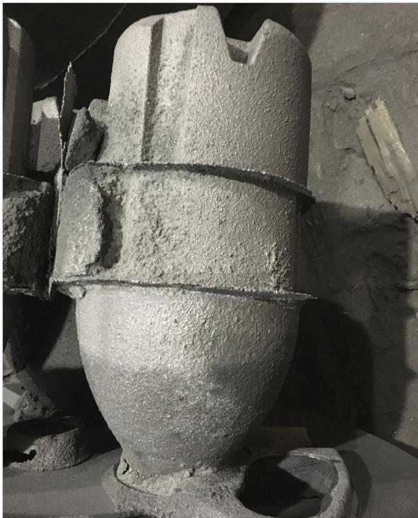
Figure 5. Cast feeder – 6.8 cm modulus
