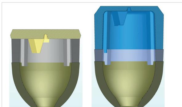
Figure 3. Basic and add-on components: 6.0 cm modulus (left), 6.7 cm modulus (right)
