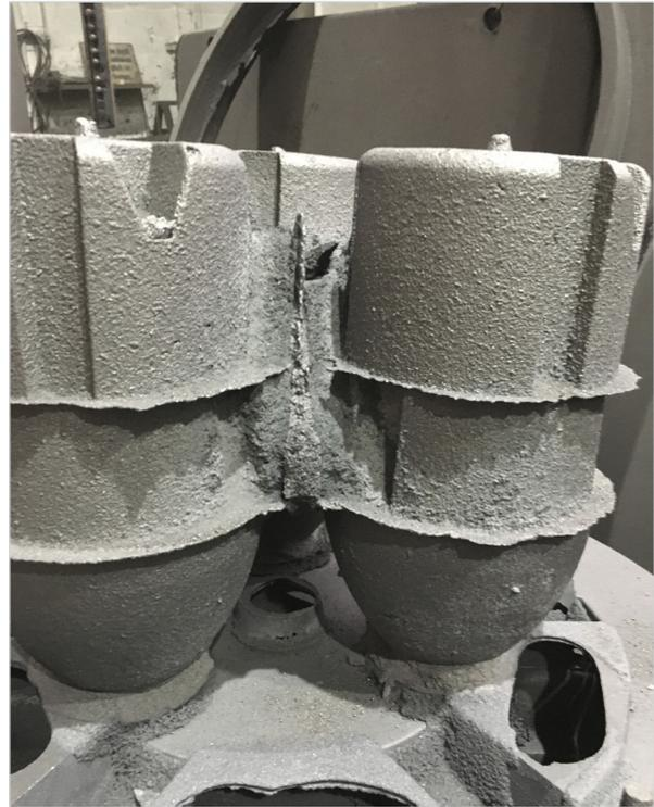
Figure 6. Feeder arrangement – three 6.8 cm modulus feeders
