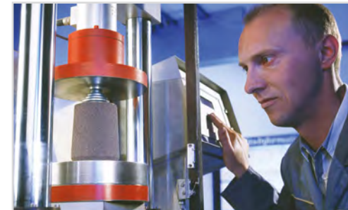
Compression strength testing of FEEDER sleeves
