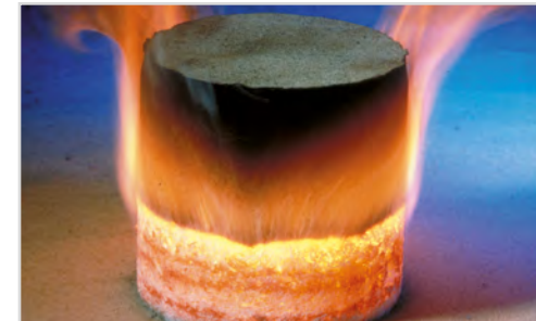
Testing burn properties of KALMINEX 2000 sleeves
