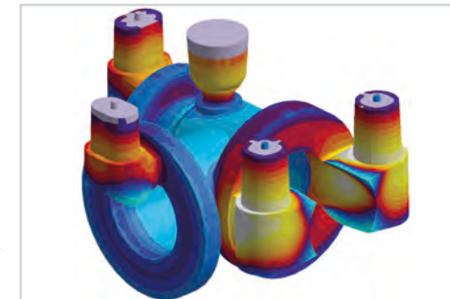
Accurate thermo-physical data allows for correct prediction of filling, solidification and feeding of the casting
