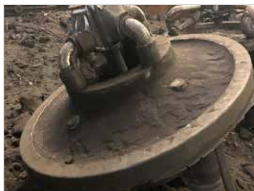
Fig. 13c: Casting with HOLLOTEX Shroud
