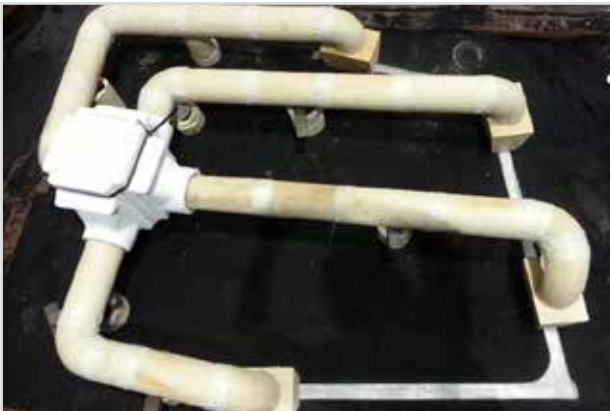
Fig. 15a: Gating system with HOLLOTEX Shroud filter box installed
