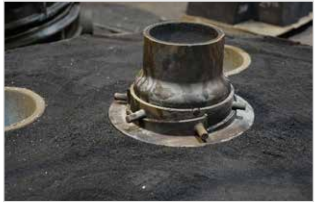
Fig. 5b: Bayonet lifting system on the top of mould
