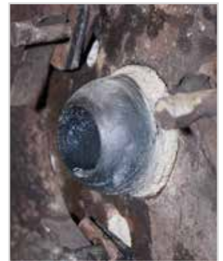
Fig. 9b: Nozzle installed at the ladle ready to use
