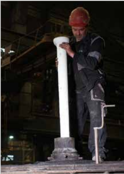
Fig. 6a: HOLLLOTEX Shroud insertion into assembled mould
