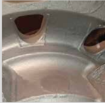
Fig. 12b: Upper casting surface after shot blasting
