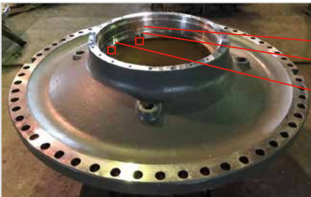
Fig. 13a: Defects after final machining
