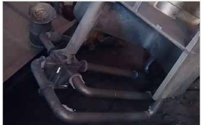
Fig. 15b: Casting with HOLLOTEX Shroud - shot blasted
