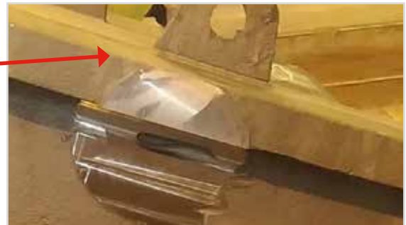
Fig. 16b: No sand inclusions or gas bubbles present
