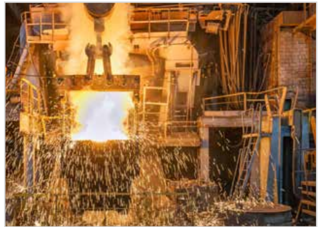
Fig. 2c: Tapping causes air entrainment and bi-films
