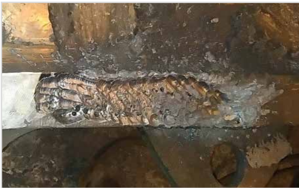
Fig. 14a: Typical gas hole defects on top surface
