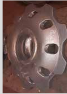
Fig. 12c: MPI after quenching
