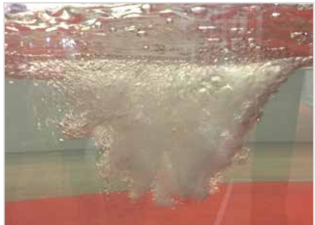
Fig. 2d: Water modelling of tapping process
