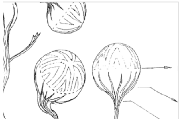
Fig. 3a: Air bubbles and bi-film trails behind
