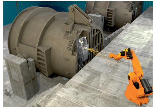
Robotized operation in ladle preparation area
