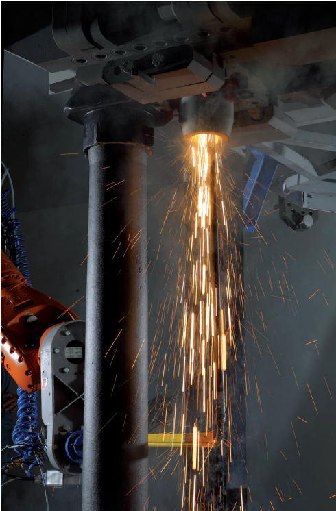
Fully automated oxygen lancing of ladle casting channel
