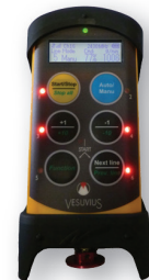
Wireless remote pendant for setting of powder discharge rate
