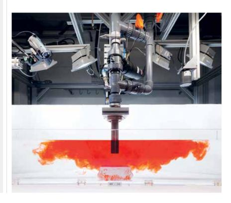
Tundish water modelling is used to optimise the design of Vesuvius' tundish solution offerings
