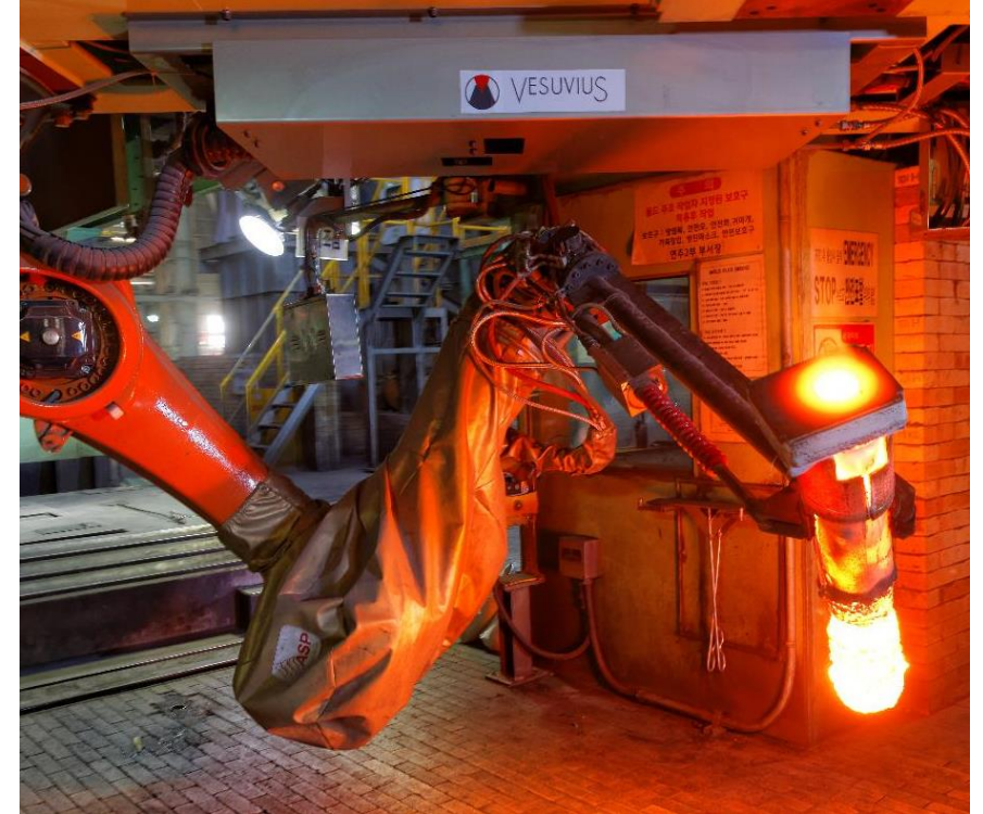
Example: Vesuvius tundish tube-change robot
