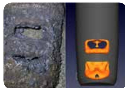
Numerical simulation of the high deposit potential region and the actual refractor nozzle after use
