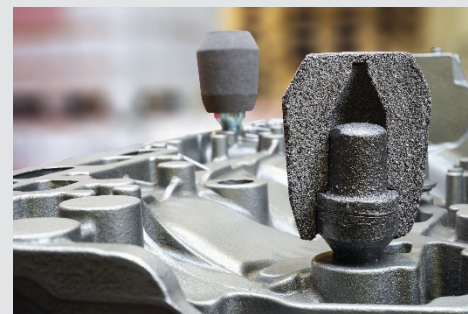
Example: FEEDEX VAK patented feeder sleeves
