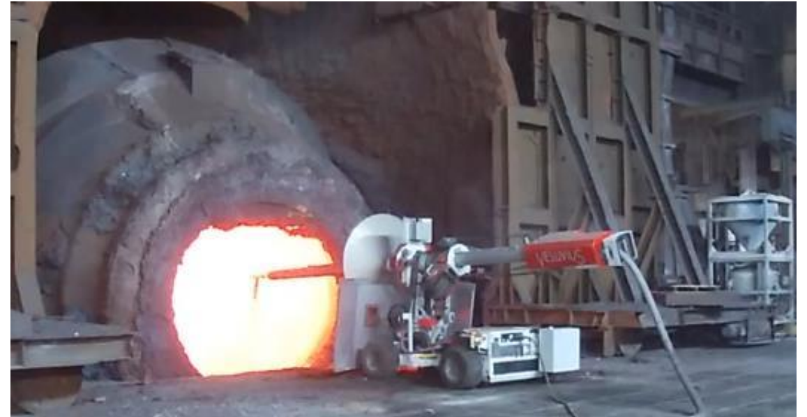
New Advanced Refractories high-speed robotic gunning solution for Basic Oxygen Furnace
